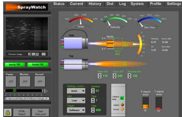
Figure 2. Temperature, particle velocity, relative flux and plume deviation measurements as shown on the SprayWatch™ system.
