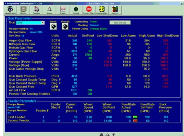
Figure 3. CITS Closed-loop process control screen.
