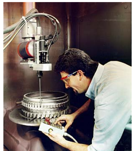
On a CNC system, the programmer uses a teach pendant to set up a fully automatic system
