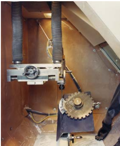
On a Semi-automatic system, the operator must set part and lance orientation manually before each batch of parts
