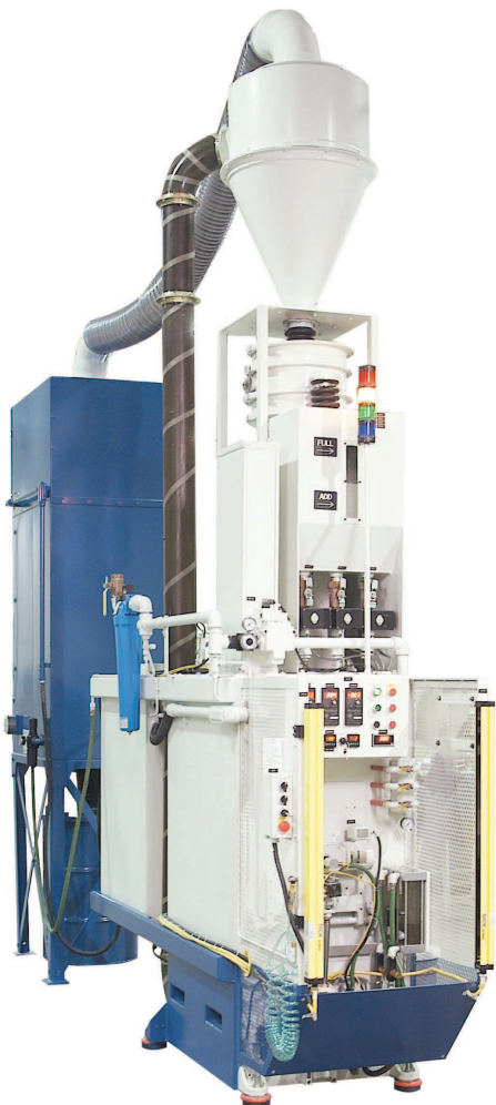
One of four turbine blade root peening machines installed at Pratt & Whitney's Turbine Module Center.
