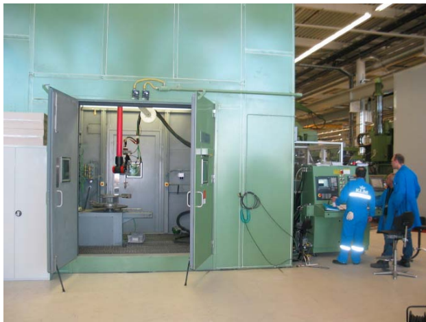
Figure 1: The new unique state-of-the-art fully automated and robotized thermal spray cabinet of Progressive Technology Inc.
